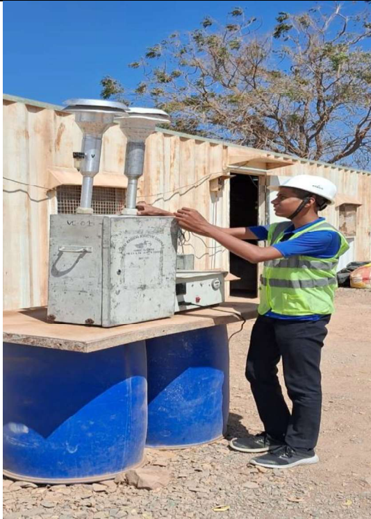
Air sampling at Upper Reservoir
