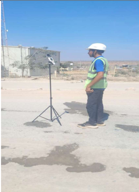
Noise monitoring at MEIL
